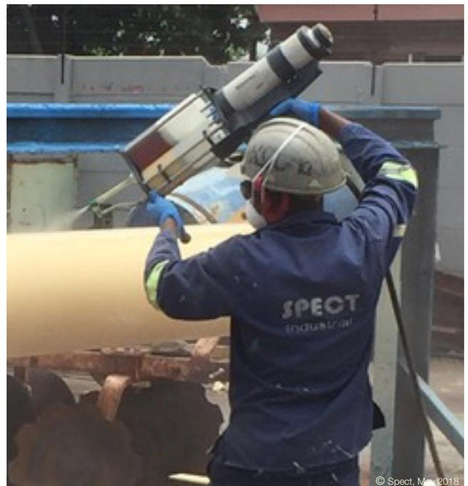
Mixpac MixCoat can even be used for coating of pipe fittings
